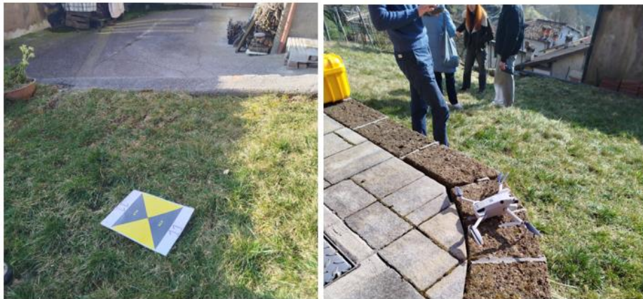
Figure 5 on the left, targets used for GPS positioning, on the right, drone
